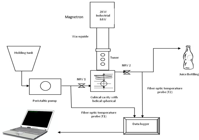
Fig 1: Continuous Microwave Heating system with specially designed applicator
